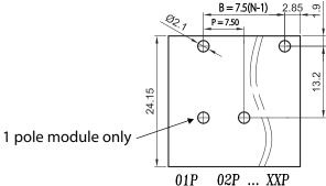
01P 02P ... XXP Recommended PCB Layout Top View
