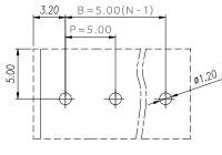
Recommended PCB Layout Top View
