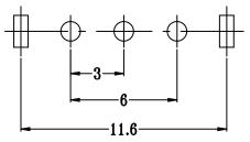
Recommended PCB Layout Top View
