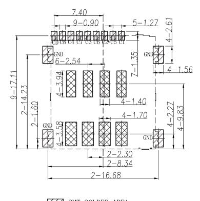
SMT SOLDER AREA COPPER RESTRICTED AREA 1. TOUCH AREA OF CONTACT TIPS NO ELECTRICAL FUNCTION 2. NO FIRST PCB\_LAYOUT CIRCUITS IN THE AREA Recommended PCB Layout Top View
