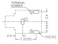
Recommended PCB Layout Top View
