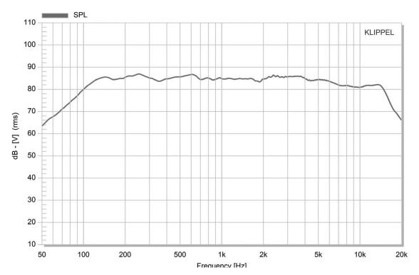
Test Conditions: 1.0 W / 50 cm on baffle
